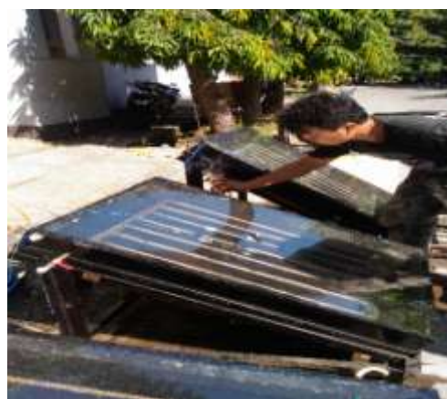
Figure 2. Photo of three solar collectors with inclinations of 15^\circ , 30^\circ , and 45^\circ .
